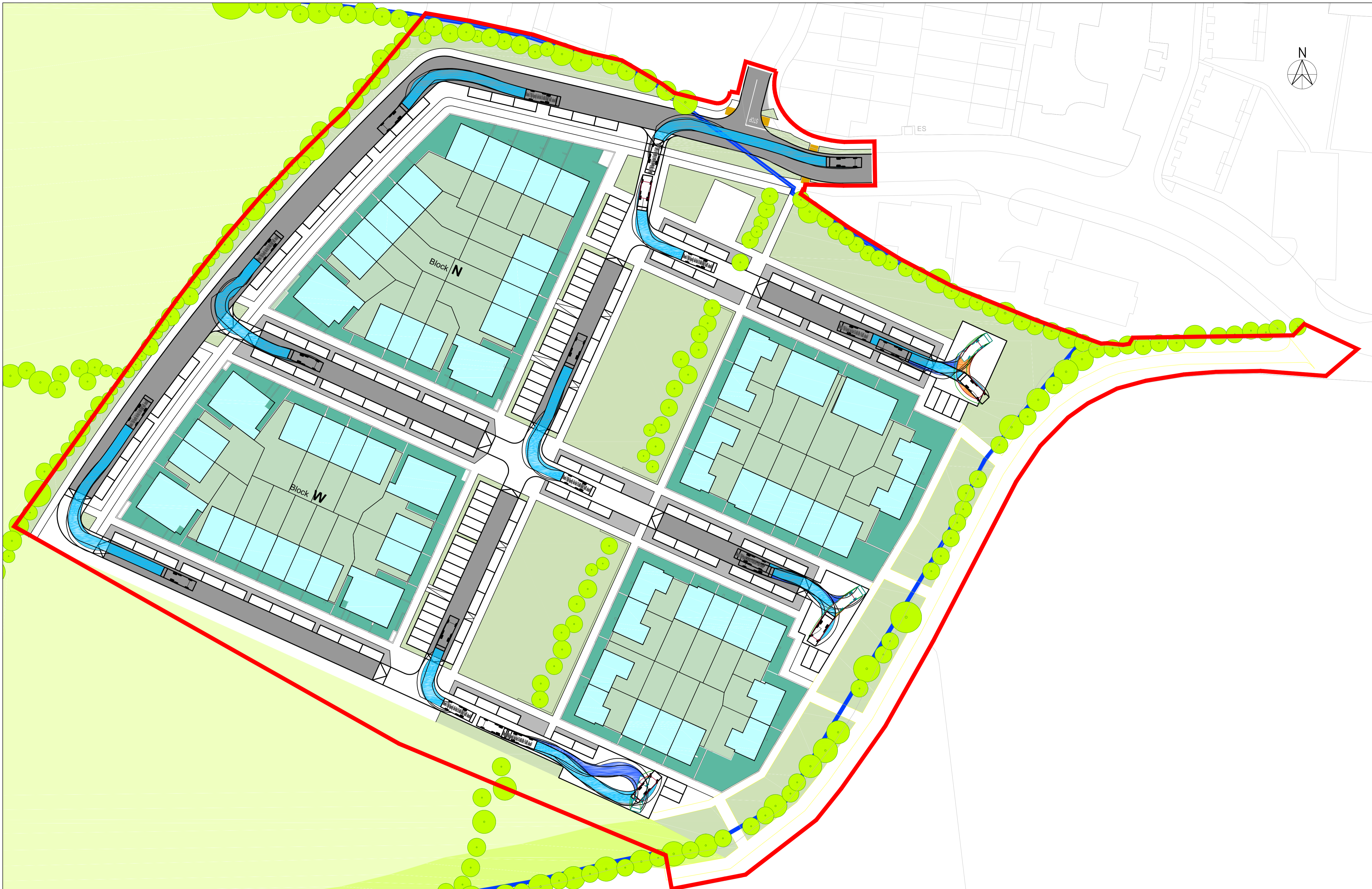
SWEPT PATH ANALYSIS FOR REFUSE TRUCK SCALE 1:500
