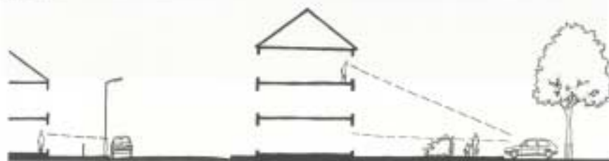
Fig 4.1 In the interests of security car parking should be overlooked by buildings where possible
